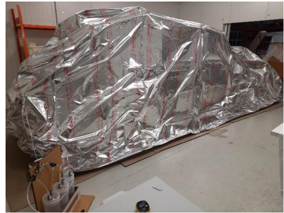
The vehicle sealed into its foil enclosure, prior to filling with nitrogen. A vacuum pump has been used to evacuate as much air as possible, to reduce treatment time and volume of nitrogen required to reach anoxic conditions. In the lower left is the simple gas humidifier used to keep humidity stable and within desired range. An oxygen alarm is in the lower foreground.
