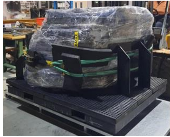
Figure 3: Coal specimen wrapped, strapped & mounted.
