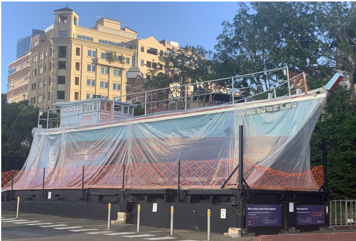
Tự Do (Vietnamese Refugee Vessel) during conservation treatment to complete structural repairs and control moisture evaporation. Image: ANMM 2022.
