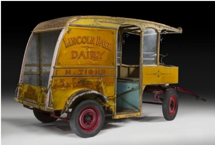
After treatment: Lincoln Park Dairy Milk cart following paint stabilisation and re-assembly. Courtesy: National Museum of Australia. Photo: Jason McCarthy
