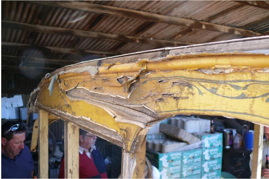
Detail showing the condition of the paint on the cart before treatment. Courtesy: National Museum of Australia Photo: Ainslie Grein
