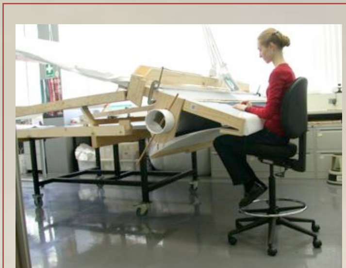
Figure 5 | Sloped work surface used to reduce muscular strain for conservator, Mary-Anne Gooden undertaking stitching.
