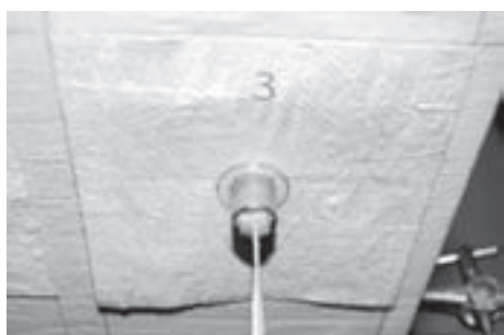
Figure 22. Bark cloth sample, Mylar™ barrier disc, magnet and weighing apparatus attached below
