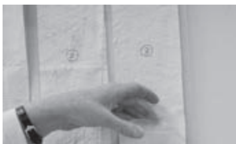
Figures 14 & 15. Loading up the bark cloth strips with lead shot in 5g increments until they fell
