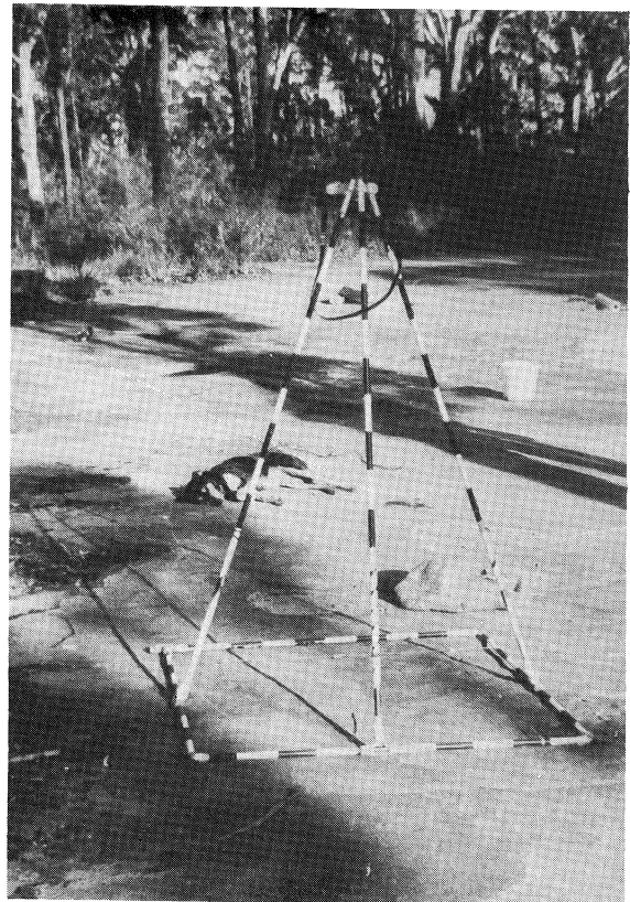
Figure 6: Tripod for low-level aerial photography. Same site as Figs. 3 and 4.
