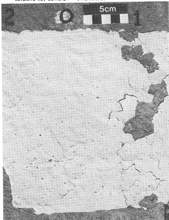
(C) Four months as above. The flaking of treatment (1) was due to a build-up of resin on the surface.
