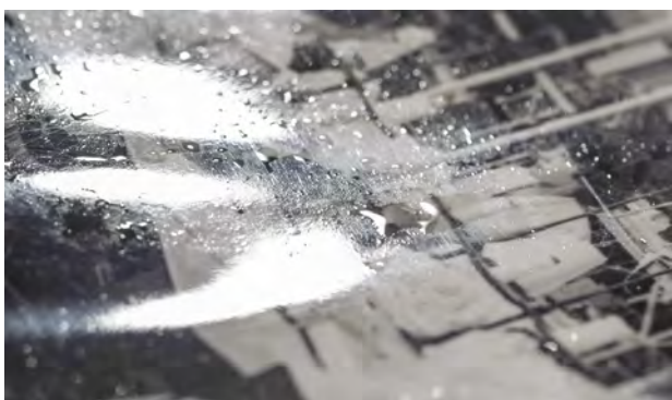
Figure 3. Visible plasticizer on the surface of the photo
