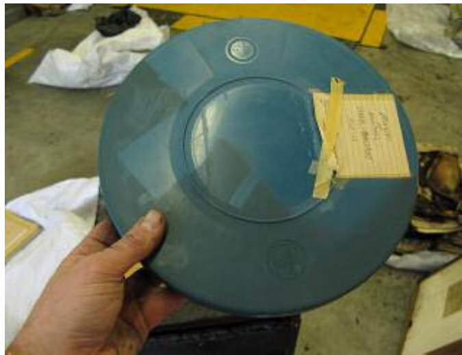
47: Film can showing brown deposit – likely fire retardant
