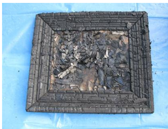
22 & 23: Wooden frame with glass that fell face-up – before and after
