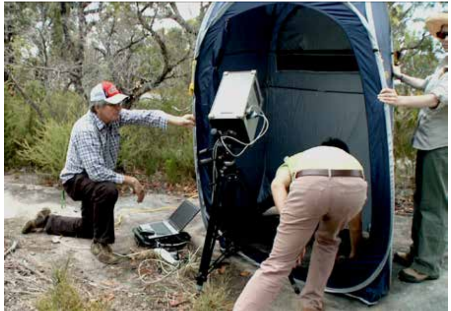
Fig 2 Laser Scanning a shallow engraving of an echidna near West Head north of Sydney. (photo – Finton Mahony)
