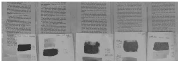
Figure 7: The lined side of the book papers and paper samples. From left to right: Tetex® applied as heat set with Lascaux® adhesive, Tetex® applied with wheat starch paste, Lens tissue applied with the mixture of wheat starch and methylcellulose, pressed between felts and Plexiglas®, Japanese tissue applied with the mixture of methylcellulose and wheat starch paste, pressed between felts and Plexiglas®, Japanese tissue applied with the mixture of methylcellulose and wheat starch paste and pressed between mountboards.
