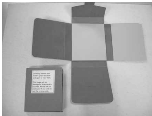
Figure 6: Rigid folder containing a damaged cased item (left) and four-flap enclosure (right). Handling instructions and specific vulnerabilities are adhered to the rigid folder.
