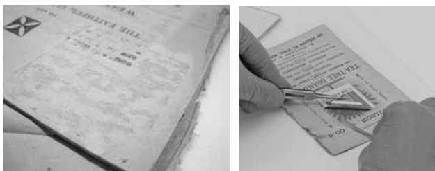
Figures 5 and 6: Removal of a barcode label, and an example of the damage left behind after removal.
