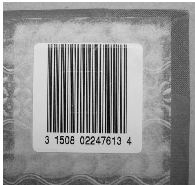
Figure 4: Barcode label is adhered to a piece of Japanese tissue which is pasted onto the endpaper.
