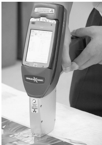
Figure 4. Innov-X Portable XRF Environmental Metals Analyzer probe.
