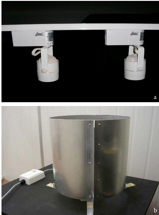
Figure 3. Light-aging devices: a) tungsten halogen component, b) fluorescent component.
