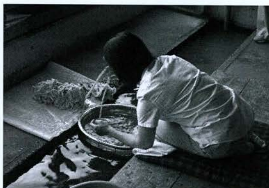
Mrs Hasegawa cleans impurities from the kozo bark in clean running water (Hasegawa Washi Kobo workshop, Mino)
