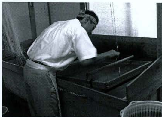
Mr Hasegawa checks the paper mould after forming the sheet (Hasegawa Washi Kobo workshop, Mino)
