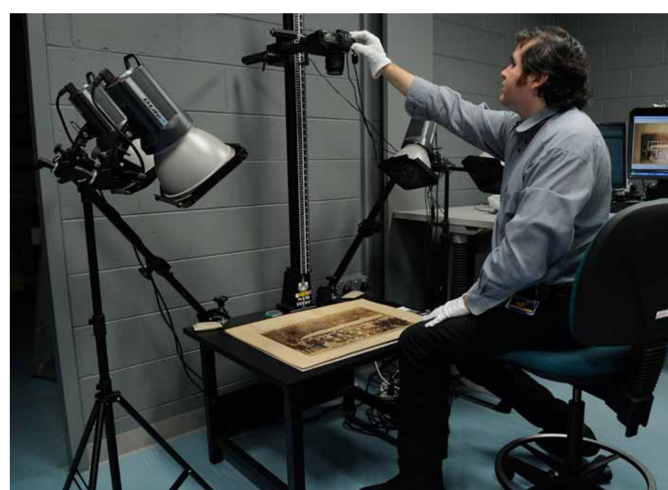
Image 2: Carrying out digitisation of the 1883 photograph using a copy stand and digital SLR
