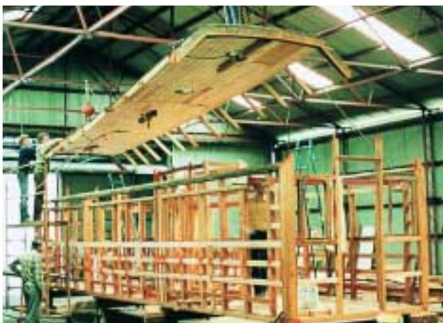
Restoration at Pichi Richi, South Australia—refitting the roof to Car No. 90, after body repairs.
