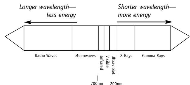
The electromagnetic spectrum with some indicative wavelengths
