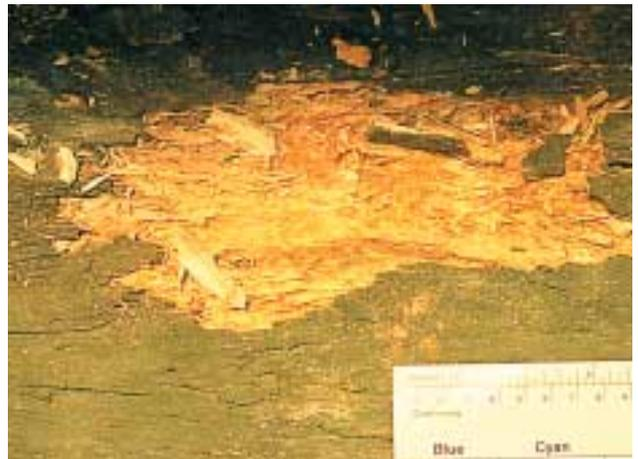
The lighter area in this photograph is an area of dry rot in a canoe.
