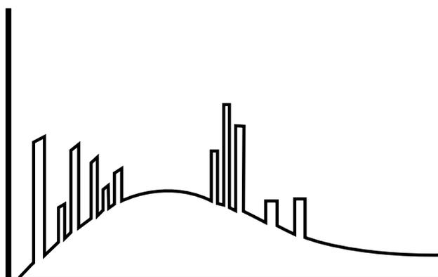
The spectrum of light from a fluorescent light tube is composed of a continuous curve caused by thermal—hot object—emission, with sharp peaks corresponding to strong fluorescent light emission at specific wavelengths. The position of the fluorescent peaks depends on the phosphors selected for the fluorescent tube.
