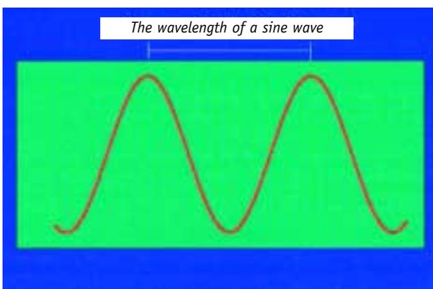
The energy in the diagram is travelling horizontally. As it travels, it moves in a wave motion passing through peaks and troughs. The distance between the peaks of the waves is called the 'wavelength' and is measured in nanometres—nm.
