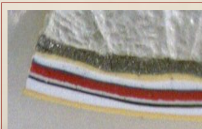
Figure 3 | Paint cross section showing yellow paint over baby poo yellow gel coat then blue, red, yellow and silver with white undercoat between layers.
