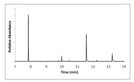
**Figure 2.** Chromatogram for the EGA-GC-MS analysis of a black polyester-based polyurethane packing foam. Peaks were identified by their mass spectrum as the internal standard hexadecane (7.85 min) and off-gassed pollutants 4-decylmorpholine (10.00 min), 4-dodecylmorpholine (11.58 min), and 4-tetradecylmorpholine (13.26 min).
