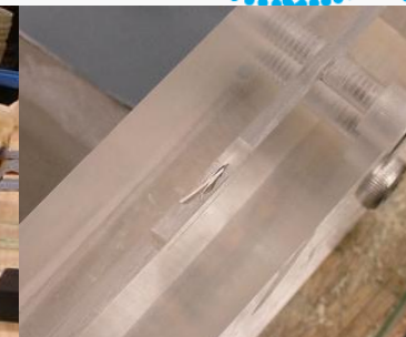
EMBEDDING THE PAINT SAMPLE IN RESIN AND POLISHING
