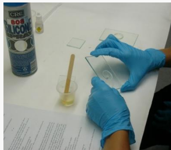
EMBEDDING THE PAINT SAMPLE IN RESIN AND POLISHING
