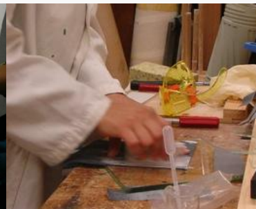
EMBEDDING THE PAINT SAMPLE IN RESIN AND POLISHING
