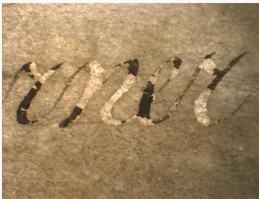
Areas of 19 th century indenture parchment document showing iron gall ink corrosion and loss.
