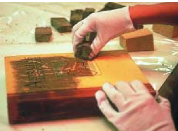
This photo illustrates the process by which soot can be removed using chemically impregnated sponges.
