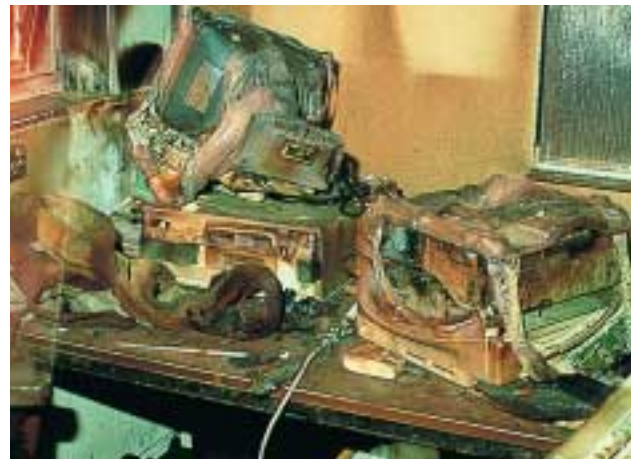
This personal computer melted during a fire in an office.
