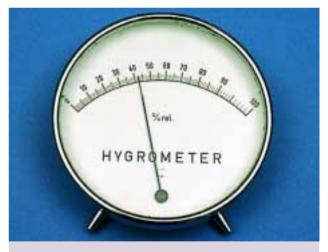
A dial hygrometer. Photograph courtesy of Artlab Australia
