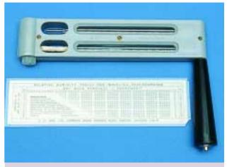
A whirling hygrometer or sling psychrometer. Photograph courtesy of Artlab Australia
